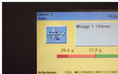
Using the In-Process "Request sample" control key lets random samples be ejected for optical packing inspections.
