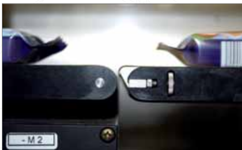
The knife-edge conveyor minimises the clearance between two belts, providing passing on the products "softer".
